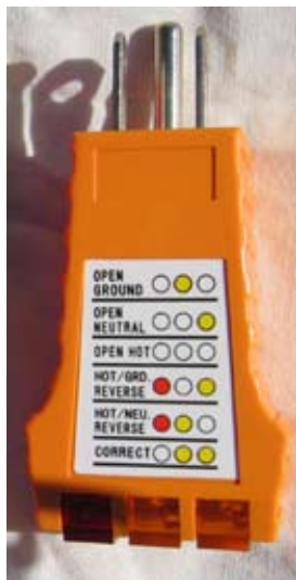
Receptacle Tester (Under $5)
